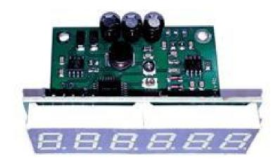
The **power supply** of the counter can be connected to a voltage of 11-14V with a current of about 500mA. If there is some noise from the multiplexer, use the following schematic to fix this:
